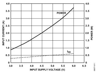
Figure 14. Typical Short-Circuit Input Current and Power vs. Input Supply Voltage, V<sub>ISO</sub> shorted to GND<sub>ISO</sub>
