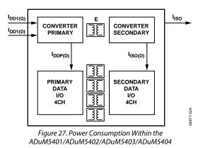
Dynamic I/O current is consumed only when operating a channel at speeds higher than the refresh rate of  $f_r$ . The dynamic current of each channel is determined by its data rate. Figure 19 shows the current for a channel in the forward direction, meaning that the input is on the  $V_{DD1}$  side of the part. Figure 20 shows the current for a channel in the reverse direction, meaning that the input is on the  $V_{ISO}$  side of the part. Figure 19 and Figure 20 assume a typical 15 pF load.
