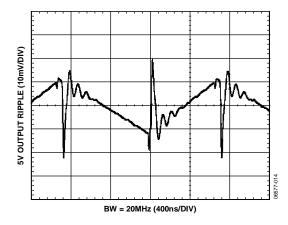
Figure 17. Typical V<sub>ISO</sub> = 5 V Output Voltage Ripple at 90% Load
