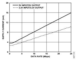
Figure 19. Typical I<sub>CH</sub> Supply Current per Forward Data Channel (15 pF Output Load)
