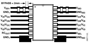
Figure 23. Recommended PCB Layout
