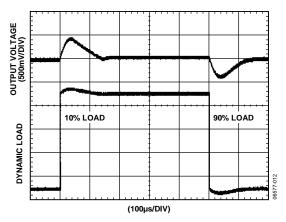
Figure 15. Typical V<sub>ISO</sub> Transient Load Response, 5 V Output, 10% to 90% Load Step
