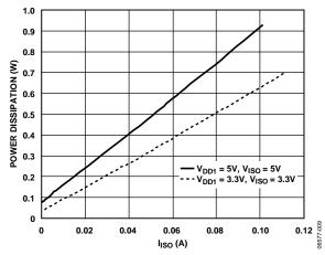
Figure 12. Typical Total Power Dissipation vs. II50 with Data Channels Idle
