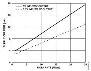
Figure 20. Typical I<sub>CH</sub> Supply Current per Reverse Data Channel (15 pF Output Load)
