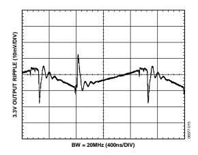
Figure 18. Typical V<sub>ISO</sub> = 3.3 V Output Voltage Ripple at 90% Load
